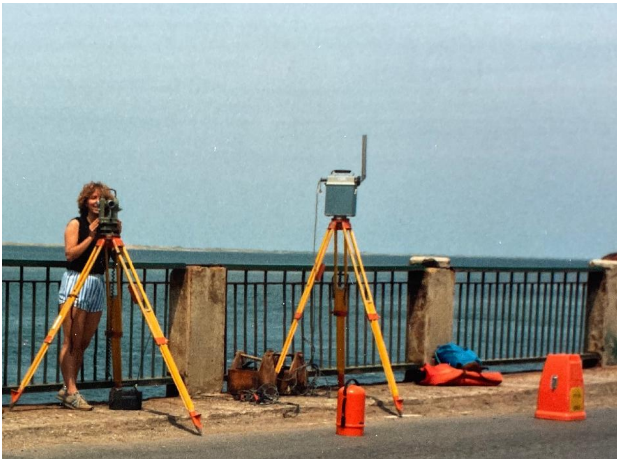
Figure 1. Student, summer 1984. Angle and distance measurements of a hydrographic launch from the bridge at Havre-aux-Maisons, Îles-de-la-Madeleine, Gulf of St. Lawrence, Quebec, Canada.
