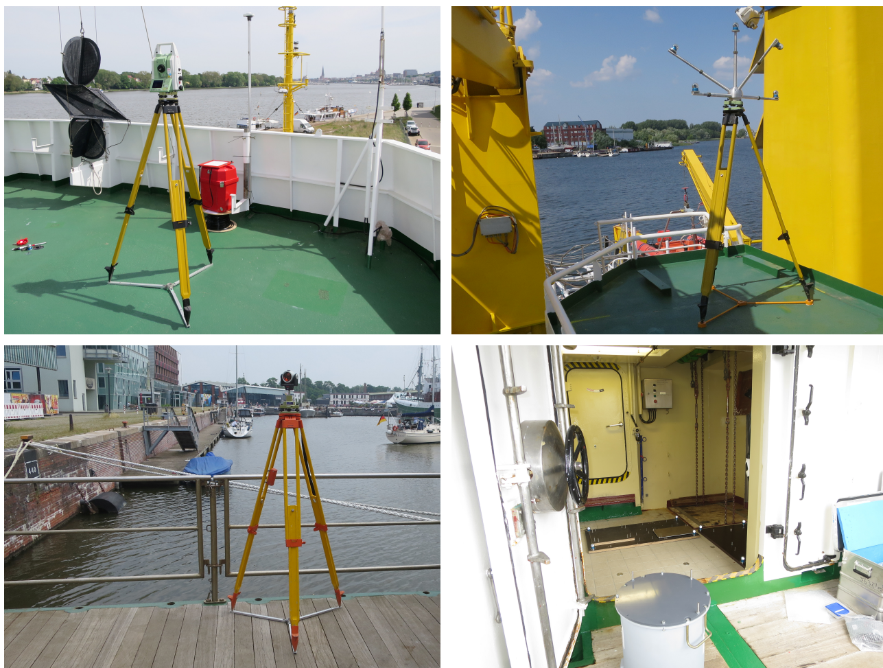
Figure 7. Local tie measurements onboard BSH's survey and research vessels VWFS DENEK and VWFS WEGA. A special array of surveying reflectors ("hedgehog") enables to transfer coordinates between the different sensors by means of 3-D transformation (top right). The gravimeter and the INS unit are referenced through the corner coordinates of their ground plates, which are determined using ball reflectors (bottom right). Photographs © Christian Lewerenz, BKG.
