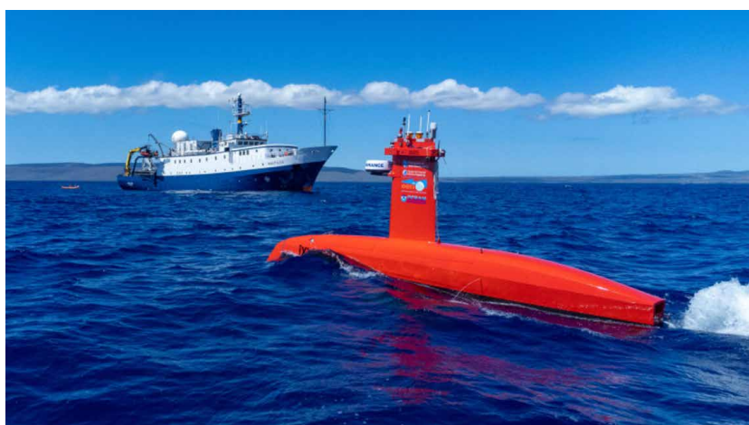
Fig. 2 The 7.7 m long DriX uncrewed vessel used by UNH as a platform to explore the applicability of uncrewed vessels to support ocean mapping and exploration missions.
