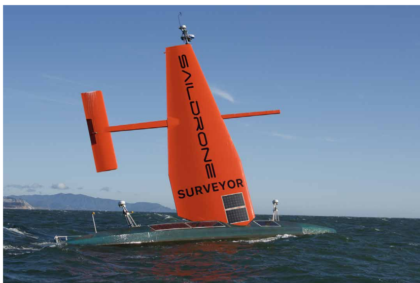
Fig. 4 The 20 m long SAILDRONE Surveyor arriving in Hawaii after a 28-day transit from San Francisco. This prototype SAILDRONE Surveyor is equipped with a 30 kHz EM-304 and 200–400 kHz EM2040, a full suite of EK-80 broadband sonars and environmental sensors as well an ESP-3 eDNA sampling system from the Monterey Bay Aquarium Research Institute.
