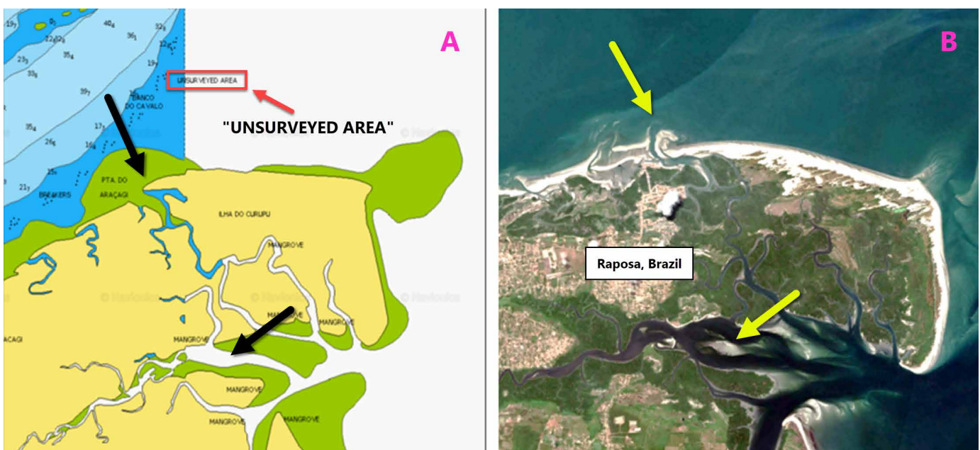
Fig. 4 Raposa, Brazil. Navionics ENC (“A”) with unsurveyed area in white. Maxar image (“B”). Black arrows in “A” and yellow arrows in “B” point to areas of visible differences between the chart and the coast.
