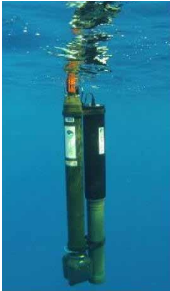
Fig. 4 The NEMO thermally recharging echo sounder float. Source: Seatrec, Vista, CA, USA.
