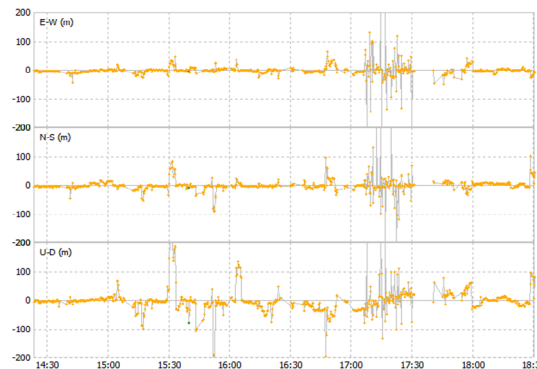
Fig. 17 Standard deviation as a function of time, for dual frequency positioning in Pracubinhas-PA.
