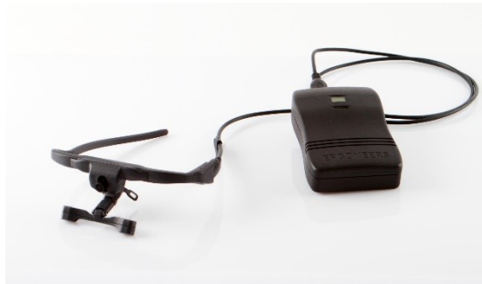
Fig. 2 Eye tracker: DG3 Dikablis Glasses 3.
