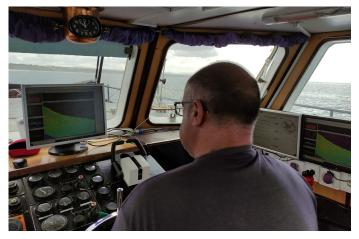
Fig. 3 Interior of the hydrographic small boat carrying out multibeam surveying (Institudo Hidrografico).
