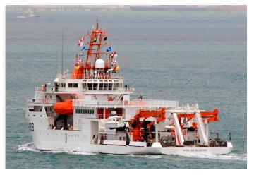
Fig. 1 Hydroceanographic Research Vessel "Vital de Oliveira" can conduct hydrographic surveys with its two hydrographic research boats and an ROV (Brazilian Navy).
