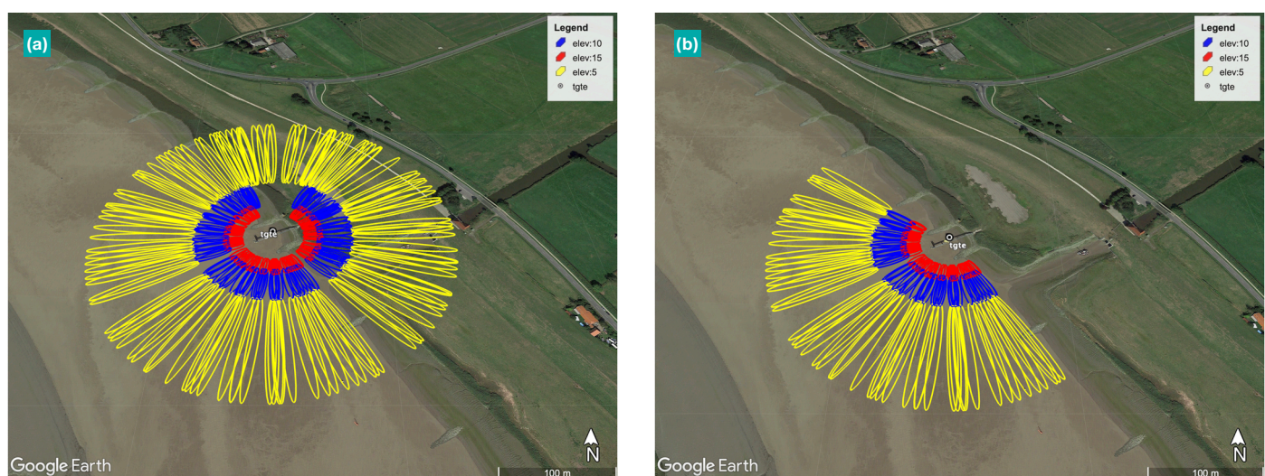
Fig. 5 (a) All potential GPS L1 Fresnel zones for Terborg. (b) First Fresnel zones after an azimuth and elevation angle mask has been applied. Reflector height taken from Table 1. Imagery created by Google Earth.
