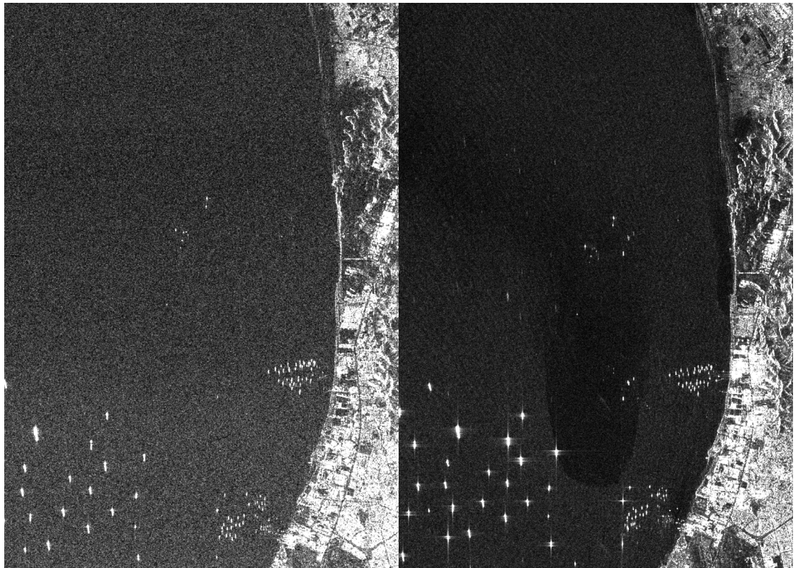
Fig. 4 Satellite image radar SENTINEL 1A, difference of polarities: VH (left), VV (right).
