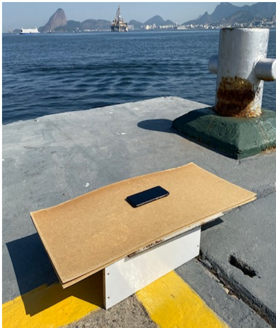
Fig. 2 GNSS data collection by smartphone.
