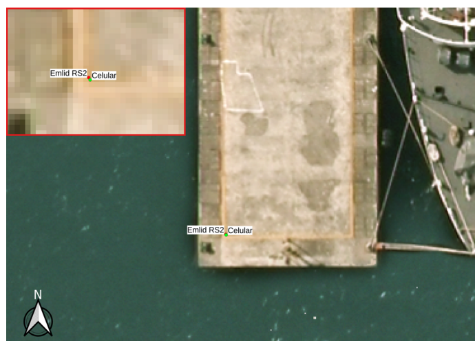
Fig. 9 Plotted coordinates of the PIRF point (Sirius – Pto Drone) using the RJNI as a reference station. Source: Adapted from QGIS (2022).
