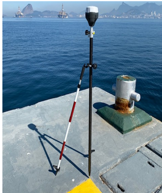
Fig. 3 GNSS data collection by high-precision tracker.
