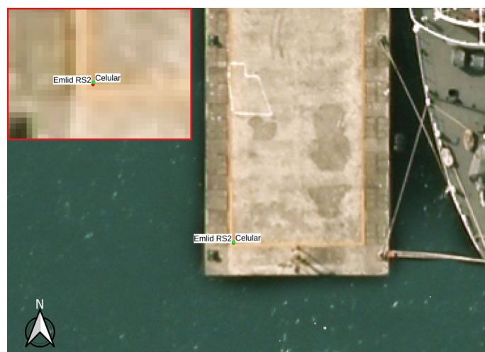
Fig. 10 Plotted coordinates of the PIRF point (Sirius – Pto Drone) using the ONRJ as a reference station. Source: Adapted from QGIS (2022).
