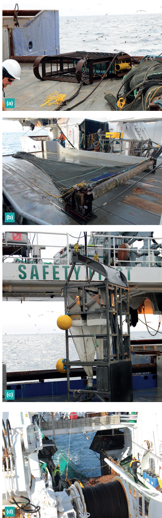
Fig. 1 Examples of (a) the NIWA seamount sled, (b) beam trawl (c) Brenke sled, (d) otter trawl. All photos by A. D. Rogers taken during The Nippon Foundation Nekton Ocean Census NIWA Bounty Trough Expedition, South West Pacific, 2024 (a, b, c) and on the RV Helmer Hanssen in Svalbard, Arctic June, 2019.
