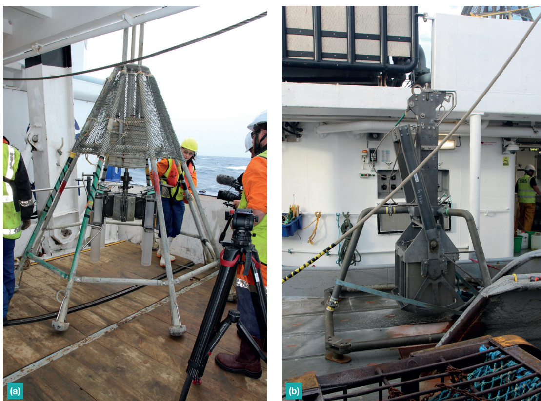
Fig. 2 Examples of (a) Multicorer, (b) Box corer. Photos by A. D. Rogers taken during The Nippon Foundation Nekton Ocean Census NIWA Bounty Trough Expedition, Southwest Pacific, 2024.
