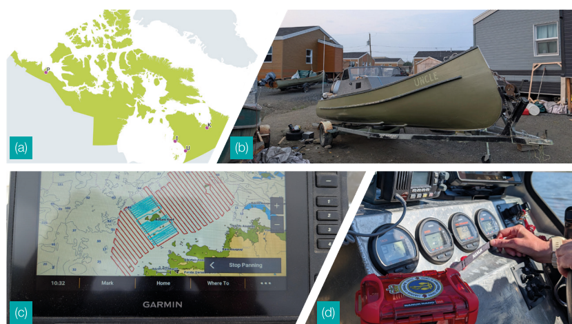
Fig. 5 (a) Locations of the four use cases: Paulatuk (NT), Inukjuak (QC), Kuujuaq (QC) and Umiuq (QC); (b) Community boat in Kuujuaq (QC); (c) Survey line pattern displayed on a community boat's fish-finder; (d) WBL 6 bathymetric datalogger.
