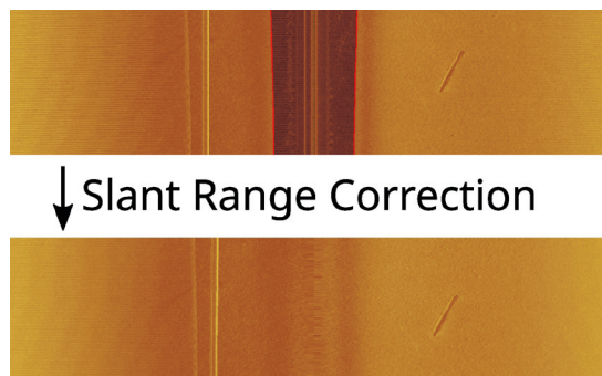
Fig. 2 Original (upper) and slant corrected (lower) data chunk. The 'seam' in the corrected data is typical for processed sidescan data and is due to the small blind area directly below the sonar transducer.
